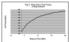
keeping what my real world rag-chew power would be. The text file ran continuously for 16 minutes. The temperature initially rose to 53 °C in 7 minutes, after which the rise slowed to less than a 1 °C/min. Spreader temperature was 62 °C after 16 minutes of continuous sending. Sixteen minutes comfortably exceeds real-world uninterrupted rag-chew or traffic transmissions.
