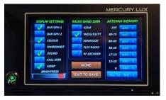
on the operating screen. Data presented includes Forward and Reflected Power, Temperature, Drain Current & Voltage, SWR, the selected Band filter, and any Warnings. Instrumented data is presented both numerically and as color bar graphs. A timer to put the display to sleep after 15 minutes of inactivity may be set. Activity or a front panel touch wakes it back up.
