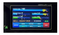
OPR/STB fault RESET, MAX FAN, and manual ANT and BANDS selections are available
